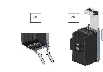
Step 3. When the fan assembly is fully home and the lower plate of the assembly has engaged with the lower mounting screws, re-tighten the mounting screws fully.
